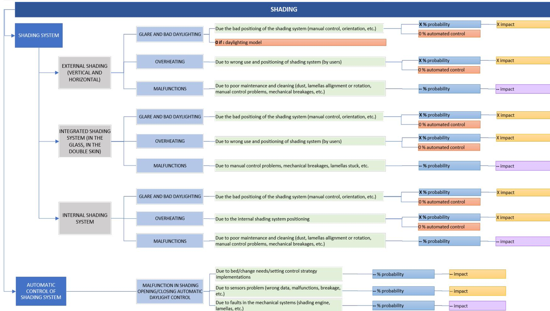
**Figure 24. Shading system risk probability breakdown definition**
